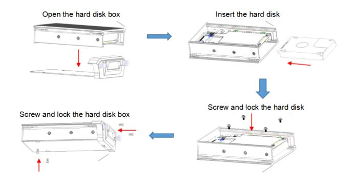
The procedure to install the hard disk of 15mm
